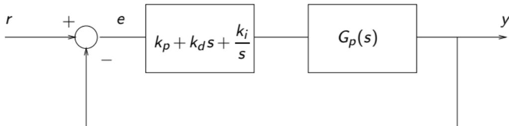
$$\frac{Y(s)}{R(s)} = \frac{(k_{hw}/\alpha)(k_d s^2 + k_p s + k_i)}{s^3 + (k_{hw}/\alpha)(k_d s^2 + k_p s + k_i)}$$
