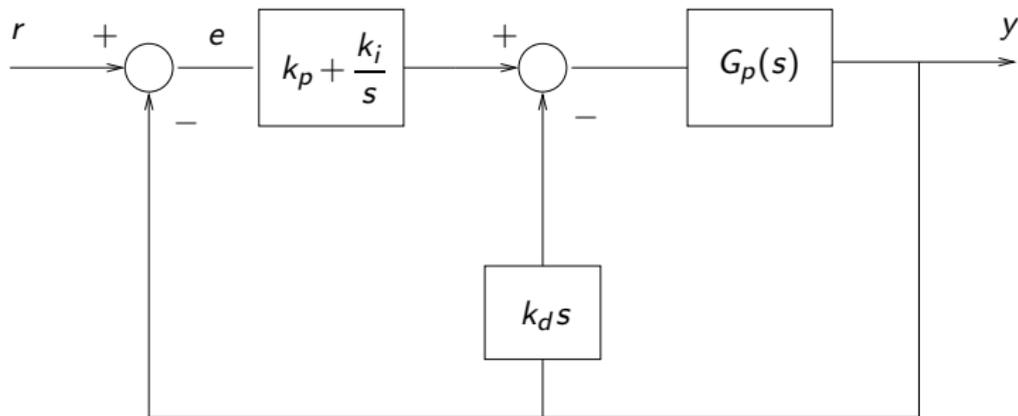
$$\frac{Y(s)}{R(s)} = \frac{(k_{hw}/\alpha)(k_p s + k_i)}{s^3 + (k_{hw}/\alpha)(k_d s^2 + k_p s + k_i)}$$
